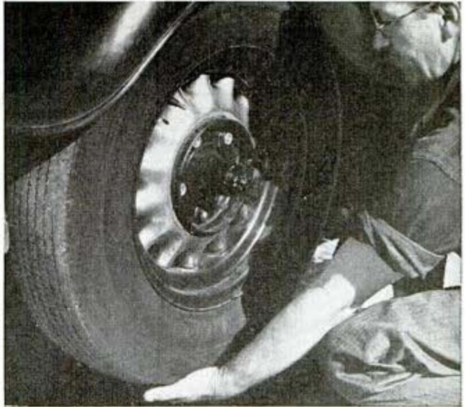
Loose front-axle bearings can be detected by trying to jiggle wheel; repack bearings every 5,000 miles and keep tight
